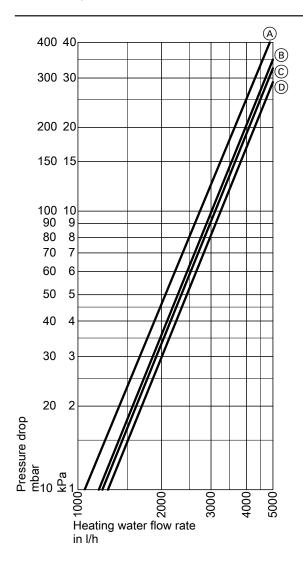
Pressure drop on the heating water side
