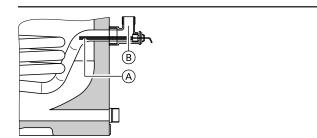
Arrangement of cylinder temperature sensor in the heating water return  $\ensuremath{\mathsf{HR}}\xspace_{s}$
